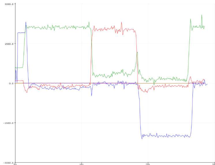
Figure 4: Triaxial readings from the accelerometer when it is held in various positions
